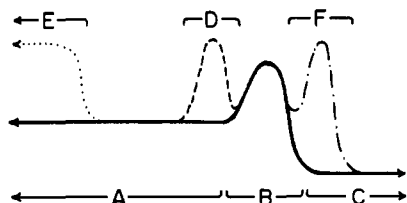
Figure 1. Representation of the potential energy surface for a gas-phase reaction, indicating regions where increases in relative energy on passing to the solid state would have different effects on the reaction rate. A, B, and C are starting material, transition state, and product, respectively. Continuation of A and C to the left and right indicates the possibility for a large region on the surface which may border transition states for other reactions. Region D is a part of A near B; region E is a part of A remote from B, but perhaps near a transition state for a competing reaction of A; region F is part of C near B.
